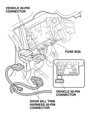
20. Attach the door sill trim harness 20-pin connector to the vehicle 20-pin connector.
