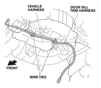
32. Secure the door sill trim harness to the vehicle harness with one wire tie.
