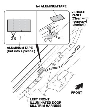
53. Using scissors, cut one aluminum tape into four equal pieces. Secure the left front illuminated door sill trim harness to the vehicle panel with one cut piece of aluminum tape.
