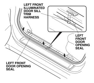
52. Using isopropyl alcohol on a shop towel, thoroughly clean the area where the aluminum tape will attach. NOTE: Do not attach the aluminum tape over any vehicle holes.
