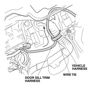
26. Align the green tape on the door sill trim harness with the hole in the instrument panel, and secure the door sill trim harness to the instrument panel with one wire tie.
