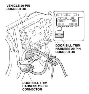
21. Attach the clip on the door sill trim harness to the fuse box.
