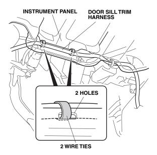
28. Attach a steel wire to the door sill trim harness with insulation tape. Route the door sill trim harness as shown.
