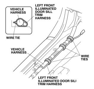
55. Plug the door sill trim harness 2-pin connector into the left front illuminated door sill trim harness 2-pin connector.
