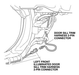
56. Bundle the excess door sill trim harness, and secure it to the vehicle harness with one wire tie.
