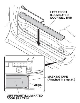
46. Attach the left front illuminated door sill trim to the vehicle panel by removing the three adhesive backings and pressing on the trim firmly with your hands.
