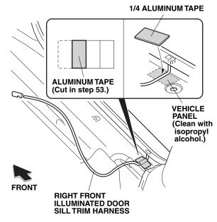
76. Secure the right front illuminated door sill trim harness to the vehicle panel with one cut piece of aluminum tape.
