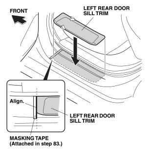
88. Attach the left rear door sill trim to the vehicle panel by removing the two adhesive backings and pressing on the trim firmly with your hands.
